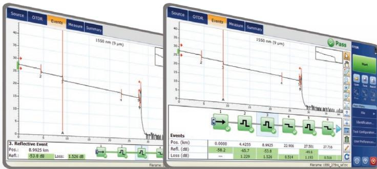
This improved linear view offers you the flexibility to display both the OTDR graph and its linear view without having to perform a toggle to analyze your fiber link.
